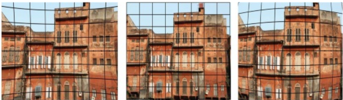
Figure 3.34: Two geometric distortion types and their correction [30]. Left: pincushion distortion. Center: corrected distortion. Right: barrel distortion.
