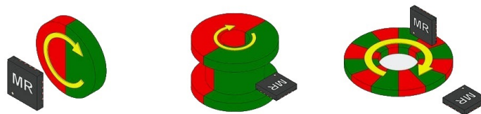
Figure 2.2: Rotation measurements by magnetic positions sensors [8]. Left: On axis angle measurement. Center: Angular measurement on circumference. Right: Two configurations of measurement of field of a pole wheel for speed sensing.
