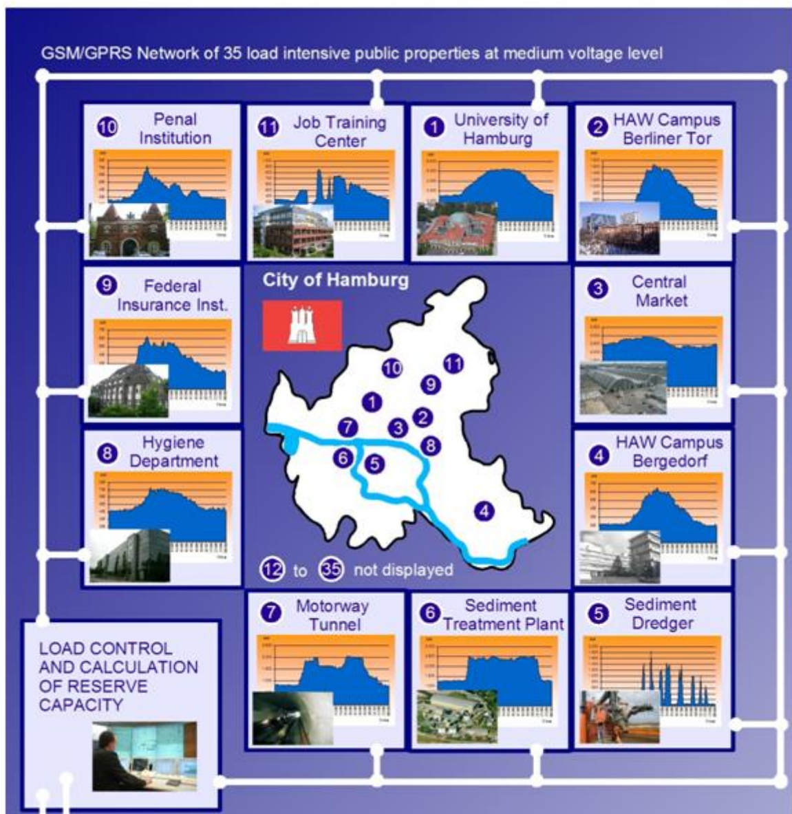
Figure 2.2: GSM/TCP IP network of MVL public properties of Hamburg includes all kinds of consumption patterns [9].
