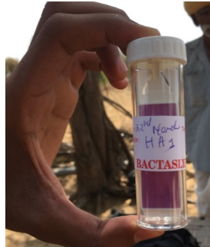
Figure 20: A labelled dipslide in its sterilized container. Image taken by the author 22.03.2017.
