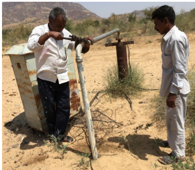
Figure 8: Tubewell 2 – Waypoint 23. Thoomba Ka Goliya. Water technician opening tubewell for collection of water sample. Image taken by the author 22.03.2017
