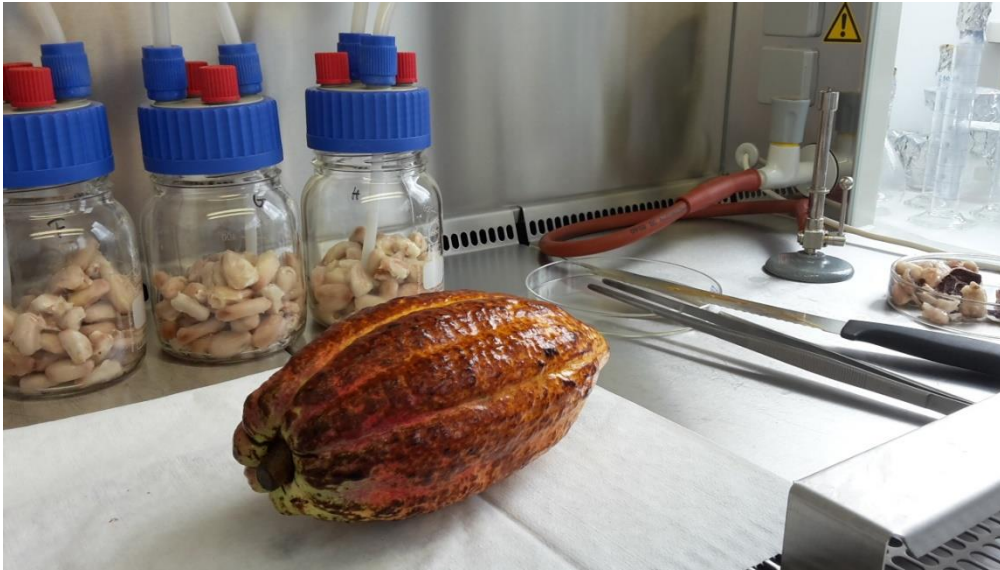
Appendix 10 pictures of fermentation-like incubation - from top to bottom- sterilized cocoa fruits and sterilized instruments under a clean bench; equally distribution of cocoa seeds to sterile glass bottles; set-up of filled incubation glasses with sterile filter in a water bath with connected nitrogen flow
