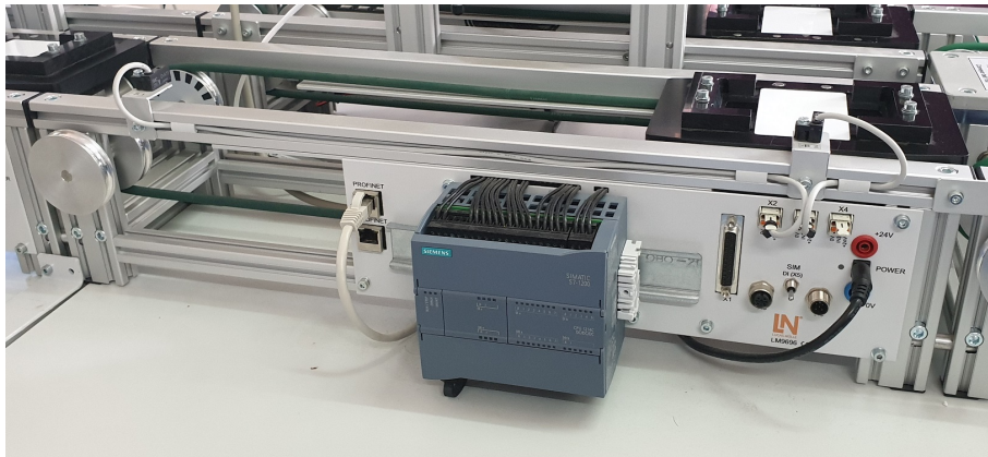
Figure 3.4: IMS1: Conveyor belt with PLC
