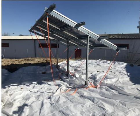
Figure 6.13. Experimental set-up for the measurements for quantifying the effect of the neighboring modules.
