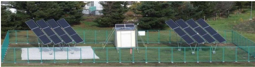
Figure 3.3 Field test site during summer. The white area of under the left array is crushed scallops’ shells [Sug13]
