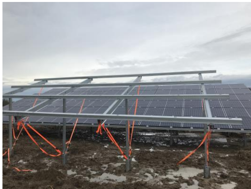
Figure 6.10. Structure used for the short-term outdoor measurements. Structure designed with four poles in the middle of the width and with four straps at each side in order to modify the tilt angle. a) without modules b) with modules.
