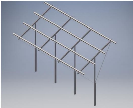
Figure 6.9. Schematic showing the structure designed to carry out the short-term measurements a) without modules b) with modules. (Enerparc AG).
