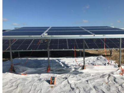
Figure 6.16. Measured bifacial gain for each module of the measurements table on a sunny day at 10:00 h.
