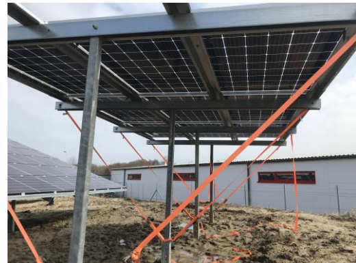
Figure 6.10. Structure used for the short-term outdoor measurements. Structure designed with four poles in the middle of the width and with four straps at each side in order to modify the tilt angle. a) without modules b) with modules.
