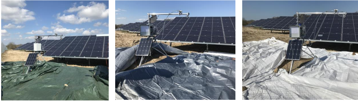
Figure 6.18. Used covers for the measurement of the effect of the albedo of the ground reflecting material and set-up for the albedo measurement.
