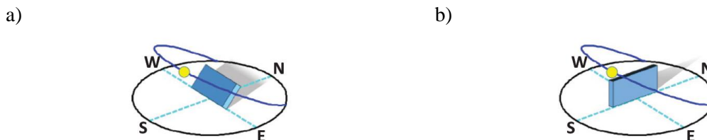
Figure 4.6 a) South facing horizontal module and b) East-West facing vertical module [Kha17]
