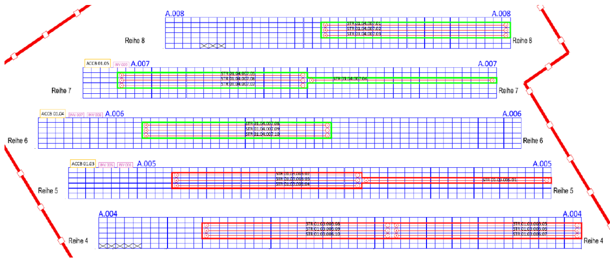
Figure 6.1. Schematic showing the setup of monofacial and bifacial modules installed at Dornstedt in Germany for the long-term measurements. Red represents bifacial modules, green represents monofacial modules (Enerparc AG).
