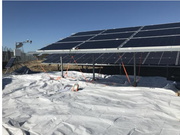
Figure 6.19. Experimental set-up for the measurements of the effect of different albedos in the bifacial gain.
