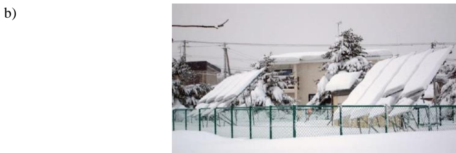
Figure 3.4.a) Field test site during winter. Both arrays are practically under the same conditions. b) Under heavy snow conditions, snow gets stacked on the surface of the module [Sug13]
