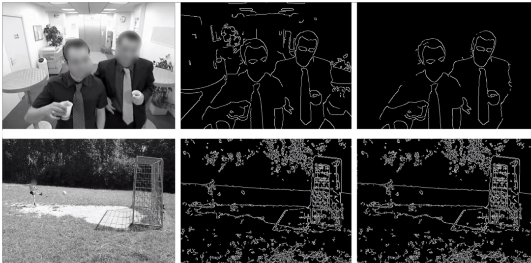
Figure 6.9: Background Subtraction implementations. Stationary (top) vs non-stationary (bottom) camera recordings
