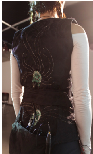
Figure 4.2: The vest transmits information for musicians during performance. The vibration elements for communication are sewn on the back of the body to look like embroidery. (Image from [18])
