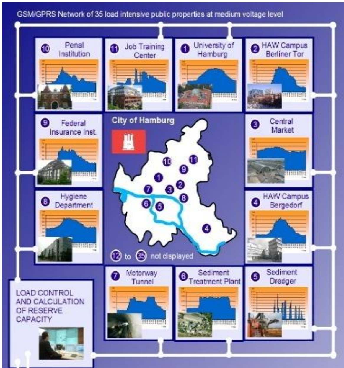
Figure 1.1: GSM/GPRS Network of 35 load intensive public properties at medium voltage level [1]
