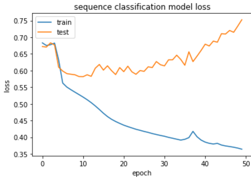
Figure 4.3: Visualization of the loss in each epoch of the sequence classifier training
