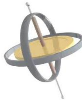
Fig. 4: Gyroscope performing a precession around the vertical [16].
