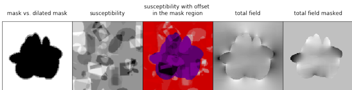
Figure 35: Creation of total field by an offset: A high susceptibility change at the boundary of the ROI was simulated by adding values of -9 to the area outside of the ROI in the susceptibility map.
