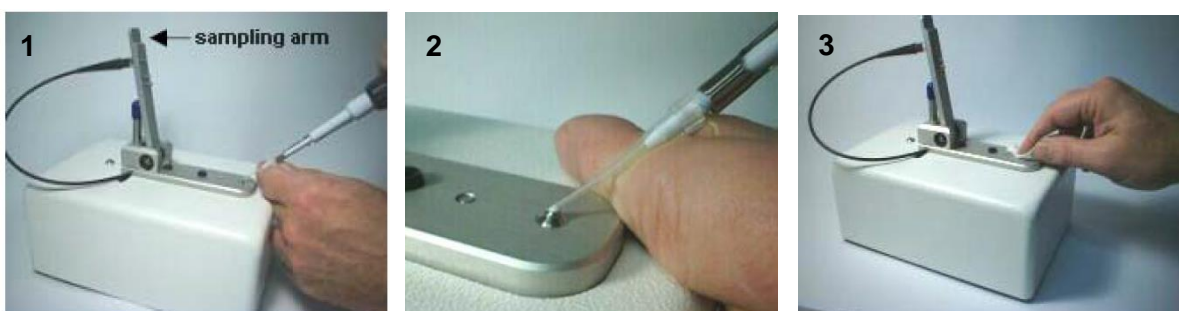
Figure 9. NanoDrop 1000 with open sampling arm with upper measurement pedestal (1), pipetting 1 \mu\text{l} sample onto the lower measurement pedestal (2). Cleaning the upper and lower measurement pedestal with soft laboratory wipe (3) (Scientific, 2019).
