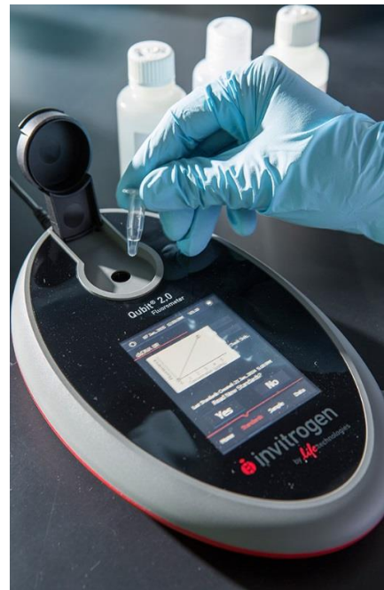
Figure 7. Qubit 2.0 Fluorescence analytical instrument, demonstration of how to insert a 0.5 ml tube (including working solution) into the sample chamber. The display shows the calibration unit (The Chinese University of Hong Kong, 2019).
