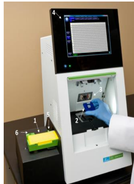
Figure 3. LabChip GX Touch, 1. 384-well plate (yellow), 2. microfluid LabChip (blue), 3. all six electrodes, 4. touch screen, 5. Ladder Tube, 6. Buffer Tube. (High Performance Electrophoresis for
