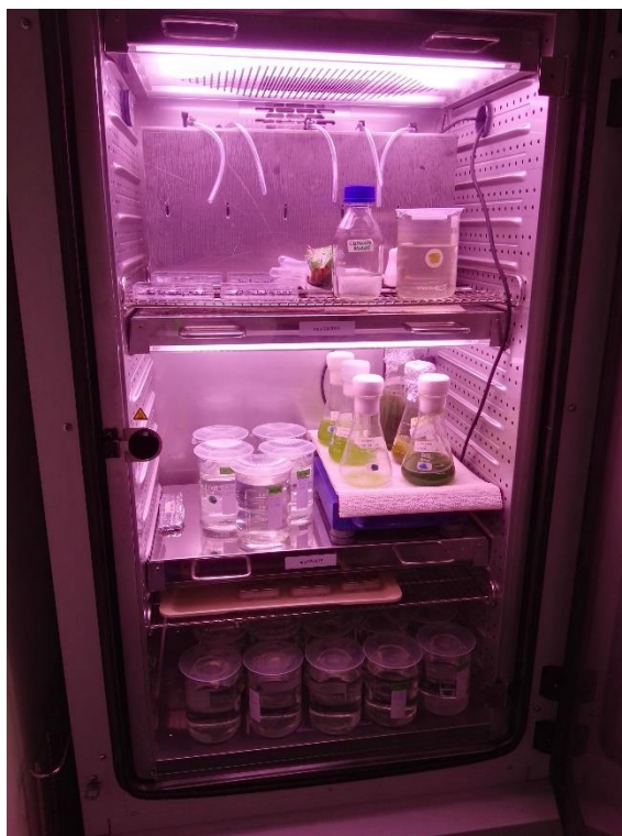
Figure 6: Incubator with constant breeding temperature and a light-dark cycle
