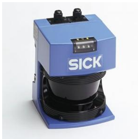
Abb. 28: Sick LMS200, 75Hz Scanfrequenz, 180°Sichtfeld, RS232/422 Interface
