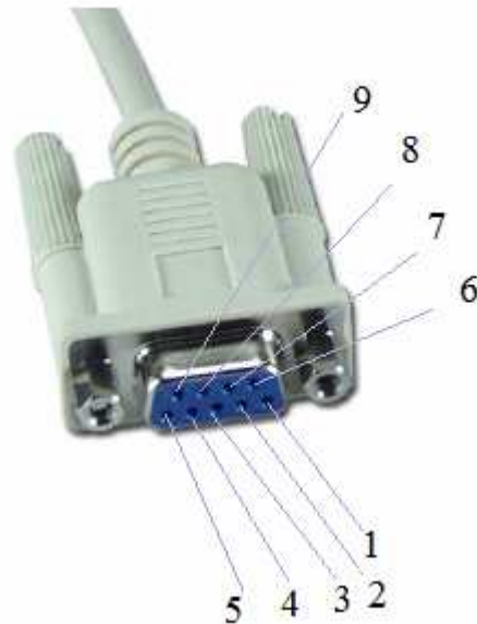
Figure 4.4.4: Female RS232 connector
