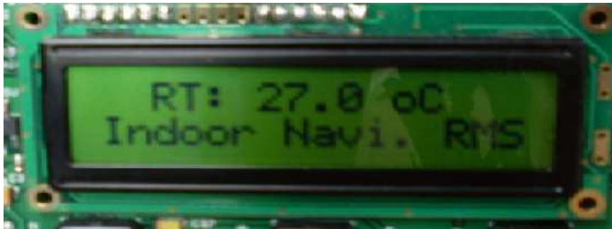
Figure 6.3.3: Room temperature (hot summer day) in °C displayed on the LCD
