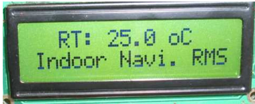
Figure 3.5.2: LCD of MSP430F169 showing displayed summer room temperature
