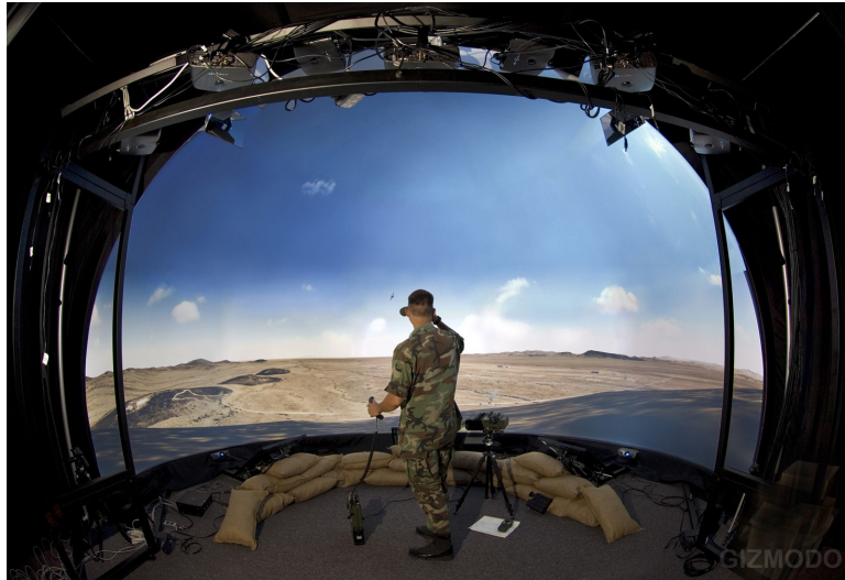
Abbildung 3.1: Ultra-high resolution multi-projector VR-System at Nellis Air Force Base in Nevada
