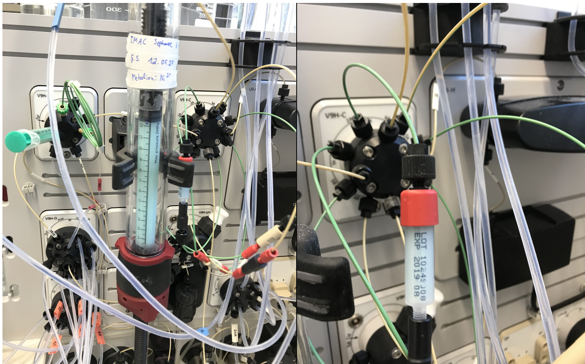
Figure 14: IMAC columns for the purification of the target protein. For the small scale purification, a prepacked column with a volume of 1 ml is used (right). Larger sample volumes are purified with a packed column (left). The bed volume of the packed column is approx. 25 ml. The chelated metal ion for both columns is \text{Ni}^{2+} .
