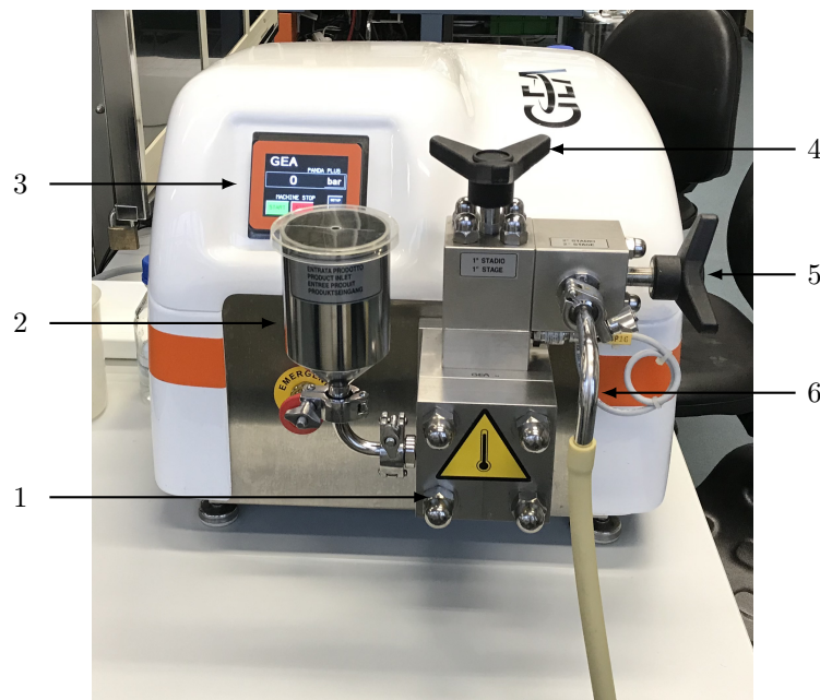
Figure 13: High pressure homogeniser Panda Plus 2000. Legend: 1. Compression block, 2. Product inlet, 3. Control panel, 4. Homogenization valve 1. stage, 5. Homogenization valve 2. stage, 6. Outlet
