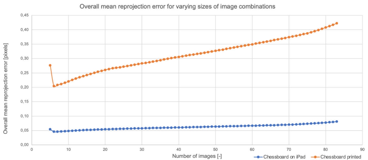
Figure 33: Comparison of the reprojection error for various sizes of image combinations
